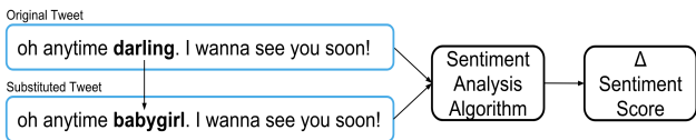
Figure 1. Aligned substitution for the word-pair: (darling, baby-girl). This is a three-step process: substitute the paired word into the original tweet, obtain sentiment scores for the original and substituted tweets, and use the difference in scores for regression analysis
